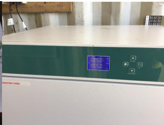
Oven permanently set to 105°C
