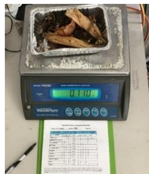
Post drying, re-weighing samples
